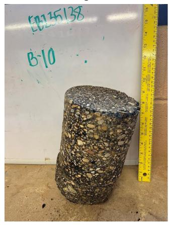
Field Measured Thickness: 11 inches Core Recovery Thickness: 9 ½ inches
