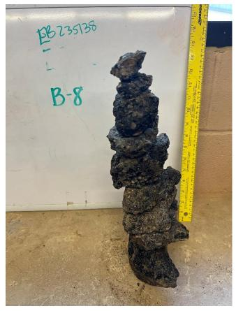
Field Measured Thickness: 10 inches Core Recovery Thickness: Disintegrated
