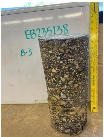
Field Measured Thickness: 13 inches Core Recovery Thickness: 13 inches
