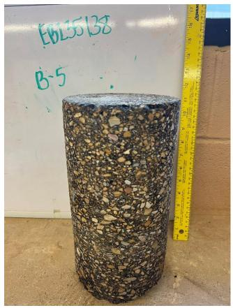
Field Measured Thickness: 12 inches Core Recovery Thickness: 11 ½ inches
