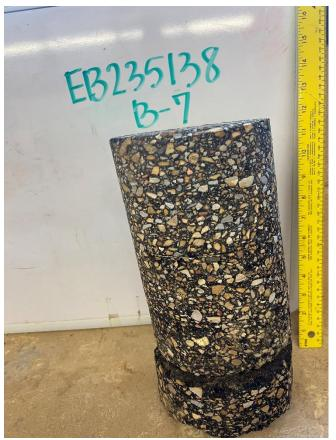
Field Measured Thickness: 12 inches Core Recovery Thickness: 11 <sup>3</sup>/<sub>4</sub> inches
