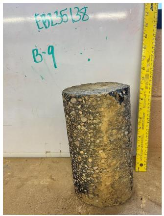
Field Measured Thickness: 11 inches Core Recovery Thickness: 9 <sup>3</sup>/<sub>4</sub> inches
