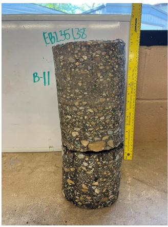
Field Measured Thickness: 14 inches Core Recovery Thickness: 14 inches
